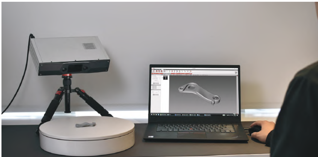
Figure 2 : Adjust the scanner and the tripod in such a way that the scanner is at a 45-degree angle looking down on the object.
